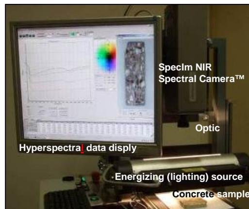
Figure 4. Particular of the architecture set-up utilized to perform a progressive and continuous concrete samples spectra acquisition based on the ImSpector™ series devices.
