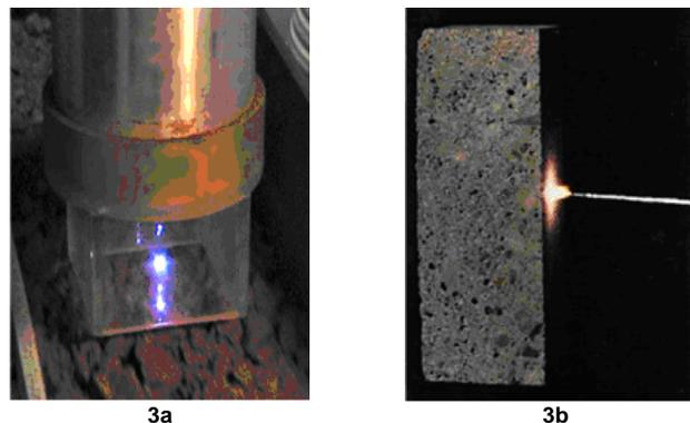
Figure 3. Examples of **Laser Induced Breakdown Spectroscopy (LIBS)**,utilized to determine the composition of stony materials on a conveyor (Honeybee Robotics, New York) (3a) and on a concrete sample (BAM, Berlin) (3b).
