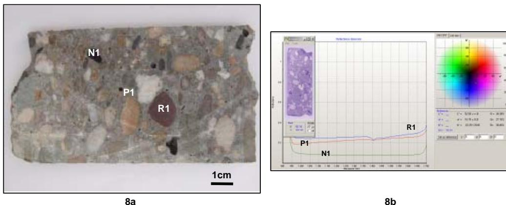
Figure 7. Example of **Hyperspectral Imaging** (HSI) based approach applied to EOL concrete core samples (4a) collected directly in the structure to demolish. The technique is adopted to identify cement (P1) and different aggregates (N1 and R1). Through the definition of a series of Regions of Interest (ROIs), it is possible, in fact, to detect the spectral signature characterizing the material inside the region defined by the ROI.
