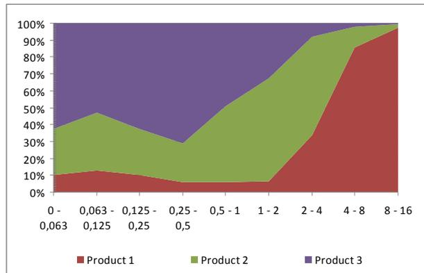
Figure 6. Recovery of mineral particles as a function of size [mm] into the three ADR products (Coarse=red, Middlings=green, Fines=blue).
