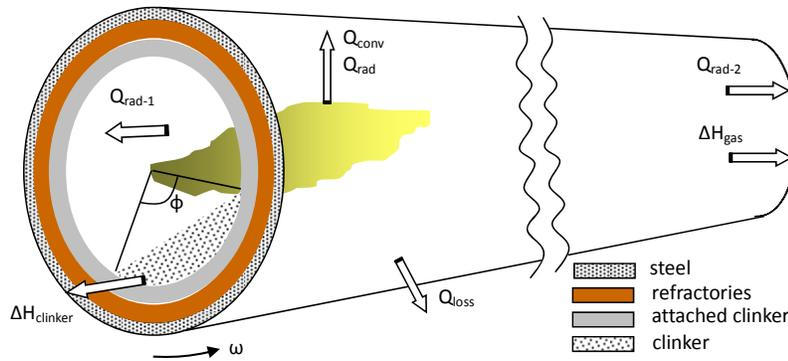
Figure 5. Schematic representation of kiln configuration indicating major heat flow components.
